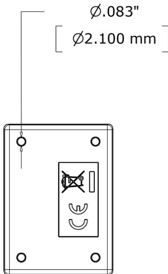
You can mount this device by removing the top half of the enclosure and using M2 bolts and nuts to secure it with the PCB still inside, and then snap the top of the enclosure back on.
