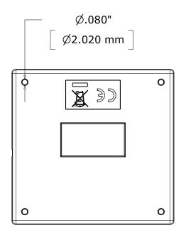
You can mount this device by removing the top half of the enclosure and using M2 bolts and nuts to secure it with the PCB still inside, and then snap the top of the enclosure back on.
