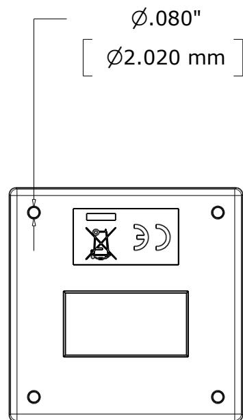
You can mount this device by removing the top half of the enclosure and using M2 bolts and nuts to secure it with the PCB still inside, and then snap the top of the enclosure back on.
