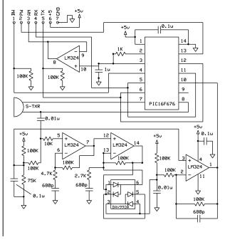
250mS after power-up, the LV-MaxSonar<sup>®</sup>-EZ1<sup>M</sup> is ready to accept the RX command. If the RX pin is left open or held high, the sensor will first run a calibration cycle (49mS), and then it will take a range reading (49mS). Therefore, the first reading will take ~100mS. Subsequent readings will take 49mS. The LV-MaxSonar<sup>®</sup>-EZ1<sup>M</sup> checks the RX pin at the end of every cycle. Range data can be acquired once every 49mS.
