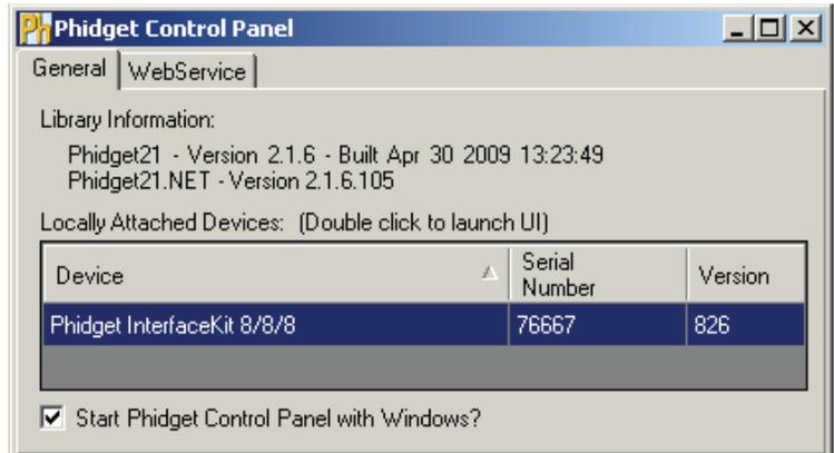
1. Double Click on **Phidget InterfaceKit 8/8/8** in the Phidget Control Panel to bring up InterfaceKit-full and check that the box labelled Attached contains the word True.
