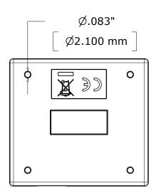
You can mount this device by removing the top half of the enclosure and using M2 bolts and nuts to secure it with the PCB still inside, and then snap the top of the enclosure back on.
