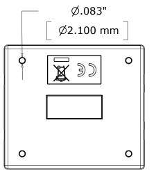
You can mount this device by removing the top half of the enclosure and using M2 bolts and nuts to secure it with the PCB still inside, and then snap the top of the enclosure back on.
