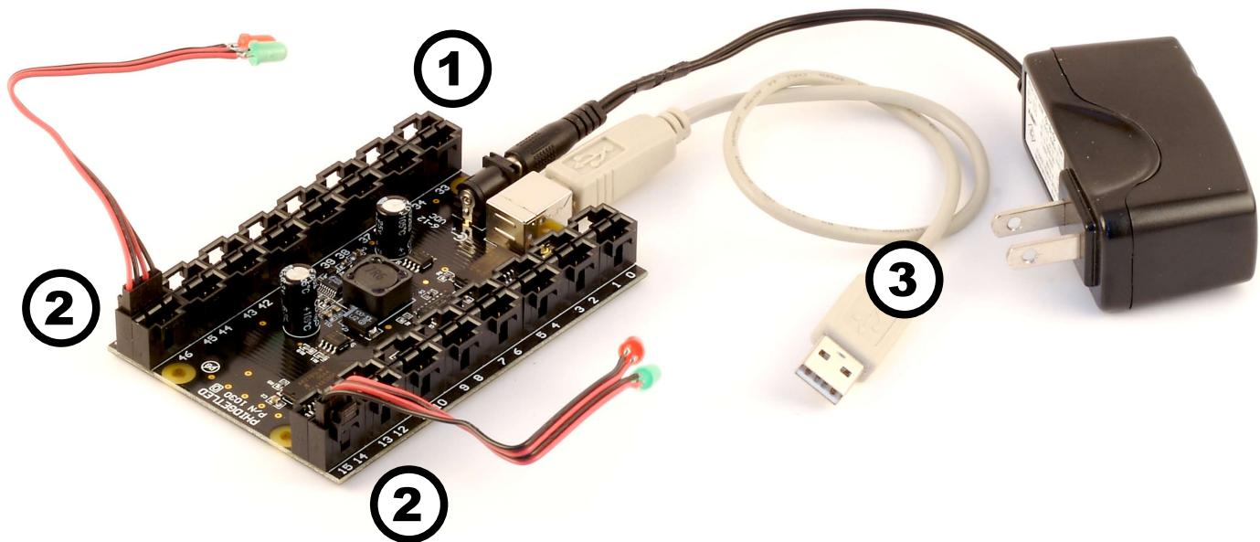
1. Connect the power supply to the PhidgetLED using the barrel connector.
