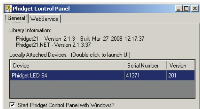
Double Click on the
