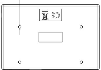
You can mount this device by removing the top half of the enclosure and using M2 bolts and nuts to secure it with the PCB still inside, and then snap the top of the enclosure back on.
