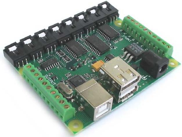
The PhidgetInterfaceKit 8/8/8 board is our most versatile Phidget, designed to be the core of a wide variety of projects. It is a USB based controller with:
