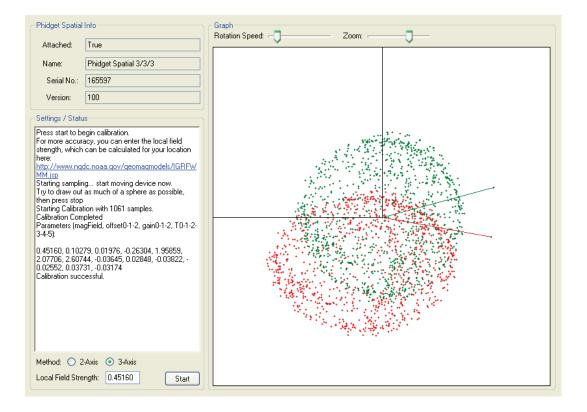
To finalize the calibration and use the results in your software application, use the resulting parameter data as input parameters to the setCompassCorrectionParameters method, in the appropriate language. This can be done once the 1056 - PhidgetSpatial 3/3/3 is attached.
