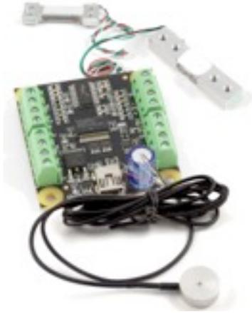
24U Phidgets Plug-In 2 has added support for the [PhidgetBridge](#) input board to read values from un-amplified Wheatstone bridges, such as strain gauges, compression load cells, pressure sensors, piezoresistive accelerometers, or compasses.
