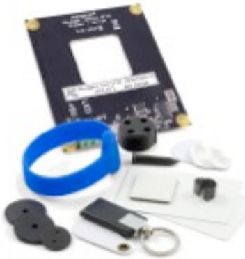
With 24U Phidgets Plug-In and the [PhidgetRFID board](#) you can read and write to RFID tags up to 6cm away. The latest board revision supports EM4100 series, ISO11785 FDX-B and PhidgetTag protocols and writes to T5577 tags.
