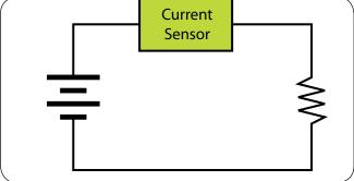
In the diagrams above, the voltage source is represented by the battery symbol. The load is represented by a light bulb or schematic resistor symbol. The current flowing from the battery to the load is measured through the current sensor.
