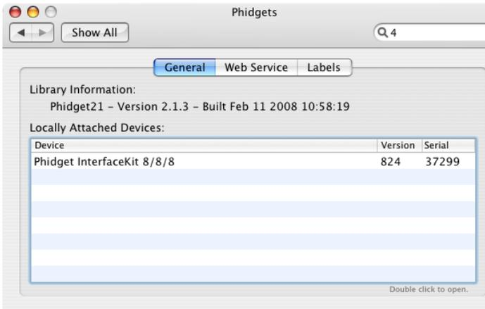
Click on System Preferences >> Phidgets (under Other) to activate the Preference Pane. Make sure that the Phidget InterfaceKit 8/8/8 is properly attached.
