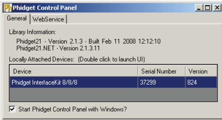
Double Click on the **Ph** icon to activate the Phidget Control Panel and make sure that the **Phidget InterfaceKit 8/8/8** is properly attached to your PC.
