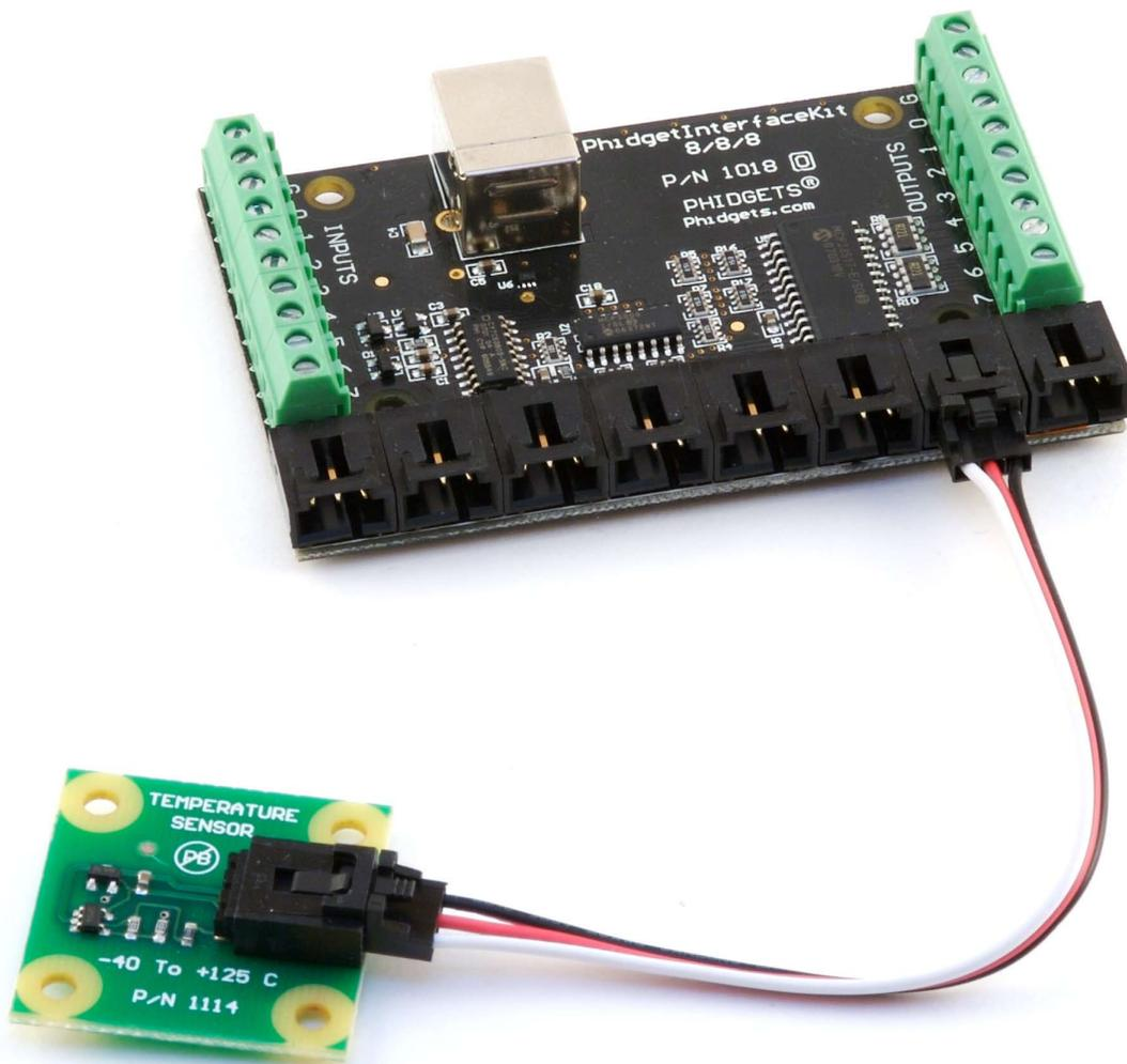
Connect the Temperature Sensor to an Analog Input on the PhidgetInterfaceKit 8/8/8 board using the sensor cable.
