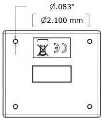
You can mount this device by removing the top half of the enclosure and using M2 bolts and nuts to secure it with the PCB still inside, and then snap the top of the enclosure back on.
