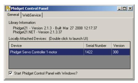
Double Click on the icon to activate the Phidget Control Panel and make sure that the **Phidget**Servo Controller 1-Motor is properly attached to your PC.
